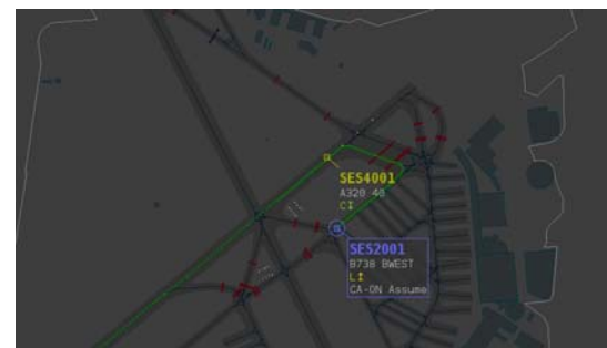
Figure 4: LUP/LND alert in SDPS display (first image), neutralized after SES4001 passes the runway entry of SES2001 (second image)
