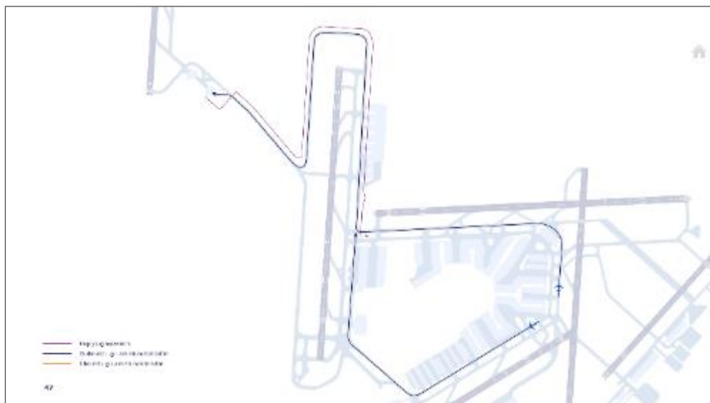
Figure 120: detailed view of an outbound route to the Polderbaan (RWY 18R / 36L) using North-bound path
