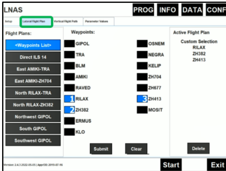
Figure 64: Definition of the waypoint sequence in LNAS for the ALBATROSS demo flights along a closed-path PBN-to-ILS trajectory.
