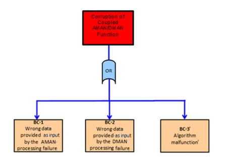
Figure 7: OH 02. Fault tree
