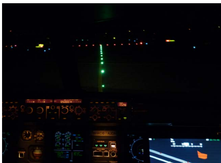
Figure 38: Activated stop bar with TCLs used for individual guidance in the foreground
