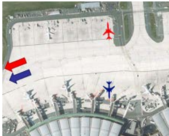
(1) Blue and red aircraft need to push back at same time and to take same exit
