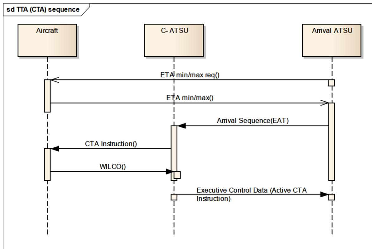
Figure 6: EAT implemented by CTA Allocation and Uplink
