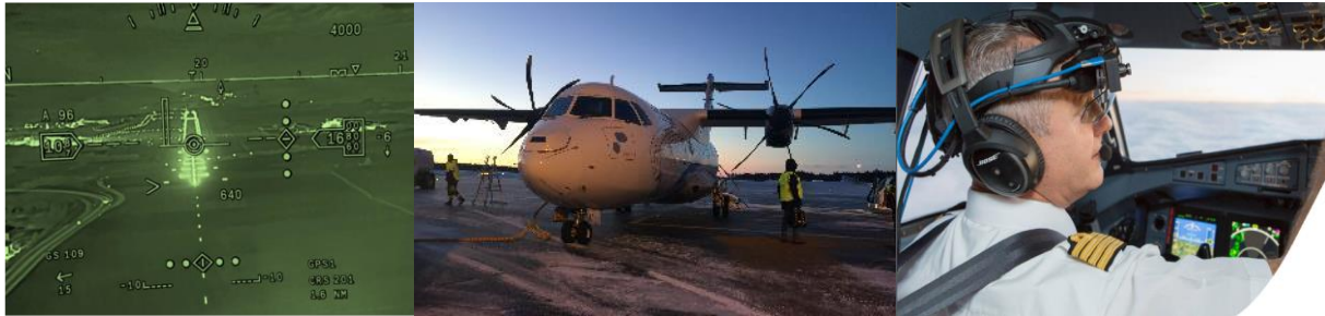
Figure 1: EFVS on ATR -600
