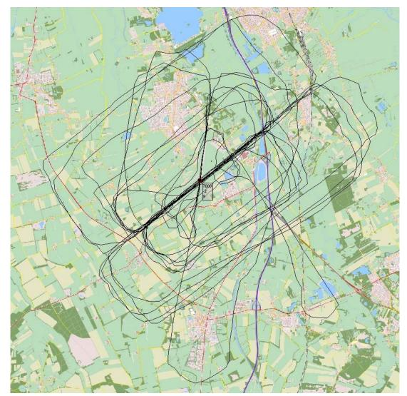
Figure 32: Ground track of VFR pattern test flight during passive shadow-mode test on Eelde
