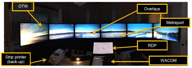
Figure 5: The demonstration platform / CWP
