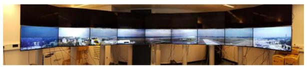
Figure 31: Single Remote Tower operation set-up for Groningen Airport Eelde
