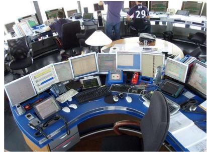
Figure 21: CDG - Tower Supervisor working position with the DMAN HMI on the left
