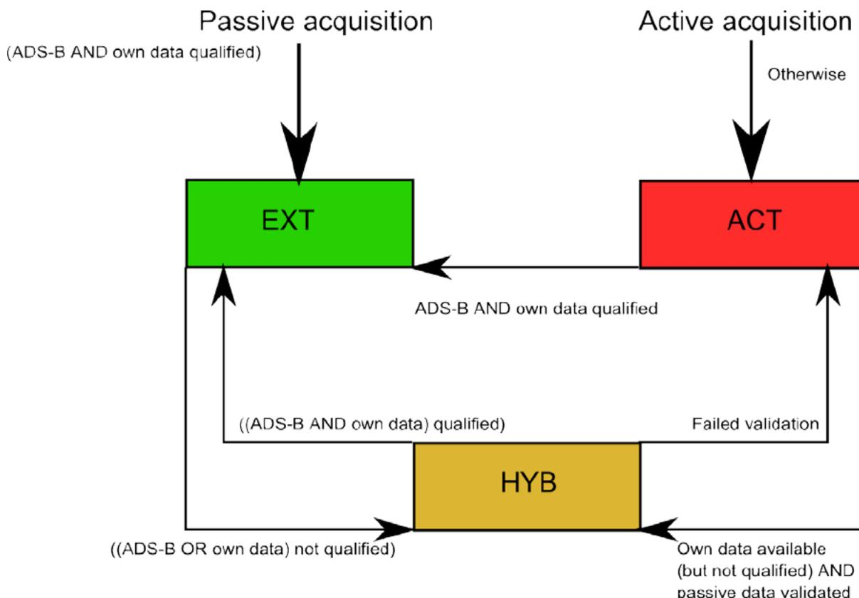
Figure 2: Transition diagram between surveillance modes when own is on ground.
