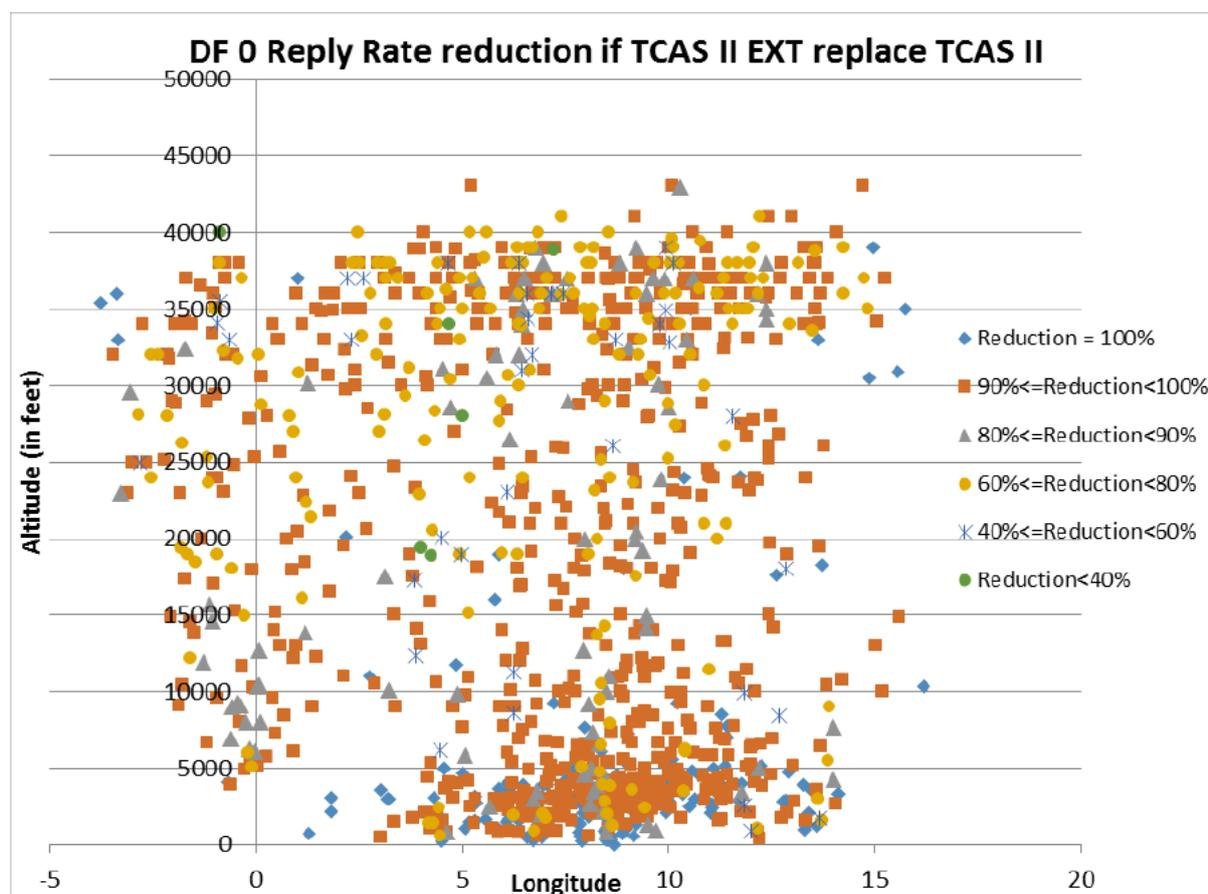
Figure 28: DF 0 Reply Rate Reduction (Vertical View)
