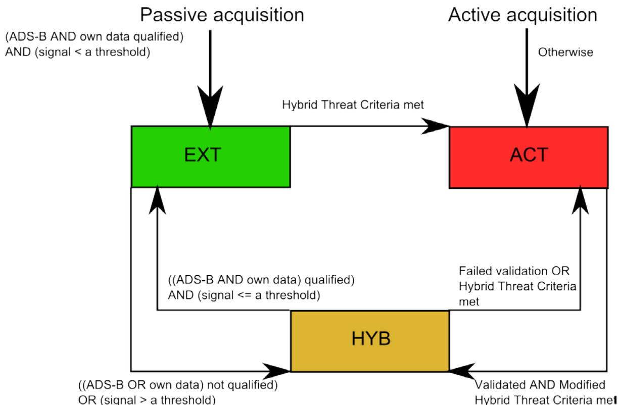
Figure 1: Transition diagram between surveillance modes when own is in the air or taking-off.
