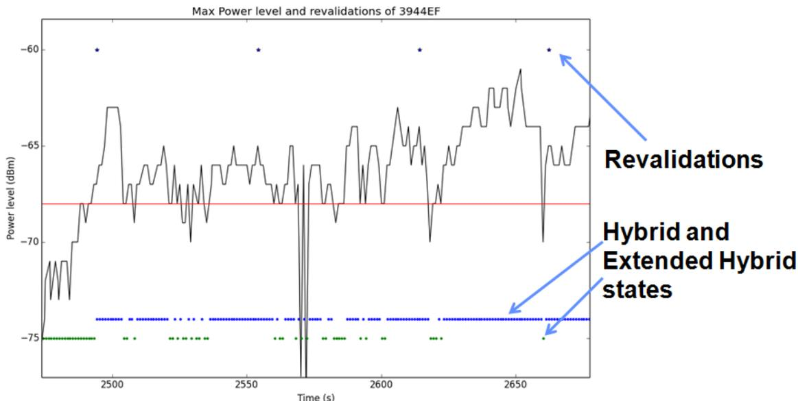
**Figure 10: Oscillations between EXT and HYB surveillance as a result of signal level variation do not lead to excessive interrogations (an illustrative example).**
