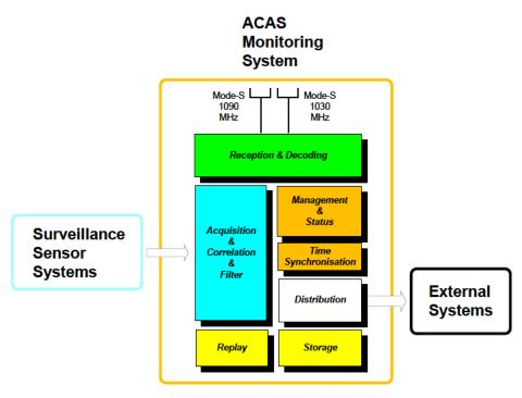
Figure 3 Main ACAS Ground Monitoring System Functions
