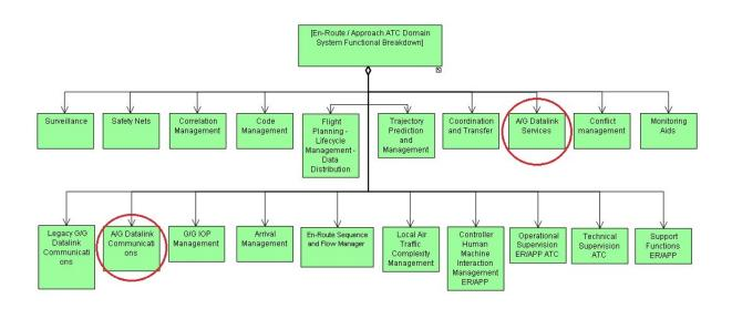
Figure 19: Functional Block Tree Diagram from EATMA
