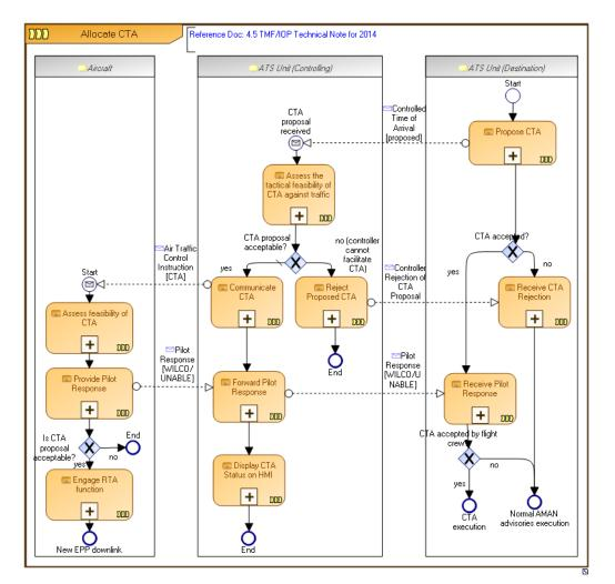
Figure 7: Allocate CTA Process Diagram
