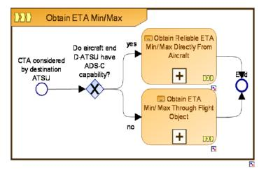
Figure 5: Obtain ETA Min/Max Process Diagram
