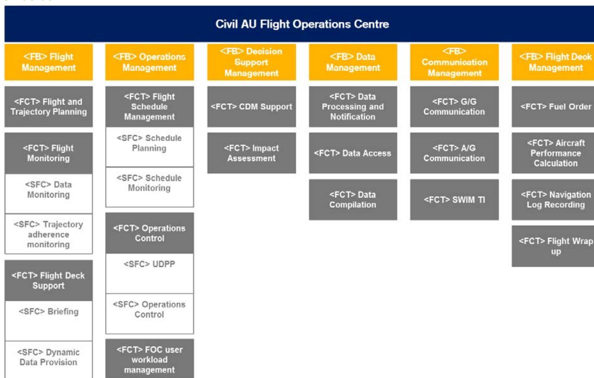
Figure 5: Function breakdown of the Flight Operations Centre
