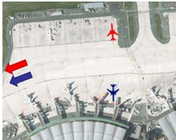
(1) Blue and red aircraft need to push back at same time and to take same exit
