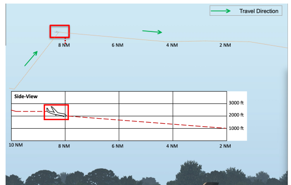
Figure 3. Illustration of an aircraft with its projected trajectory (side view) and the corresponding vertical profile (top). At approximately 8 nautical miles, the aircraft makes altitude adjustments before reaching the final approach fix, resulting in increased errors in position estimation.
