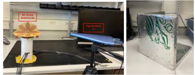
Figure 11. IEFT plot: Lab picture with the Yagi antenna at the TX and the 3D VA at the RX. Left: LOS scenario; right plot: Obstacle used for NLOS scenario in the wave path.
