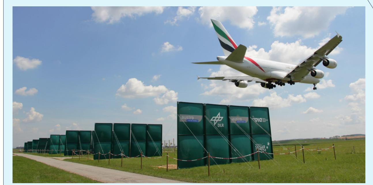
Pre-industrialisation of wake vortex decay enhancing devices (plate lines, PJ.02-01-07) is demonstrated at Vienna Airport, showcasing increased safety levels and aircraft separation reduction potential.
