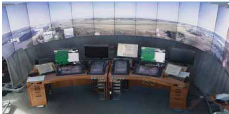
Figure 1 VR visualizations from the remote tower control center at Sundsvall airport in Sweden
