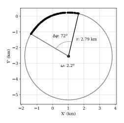
Figure 7. Computation of turn radius and turn rate for an example trajectory
