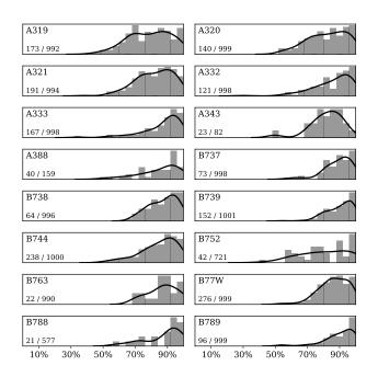
Figure 15. Distribution of maximum flight mass per aircraft type (only  $m < m_{\rm mtow}$  are considered,  $C_{L,max} = 1.4$ )
