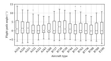
Figure 9. Distribution of flight path angles during the turns per aircraft type
