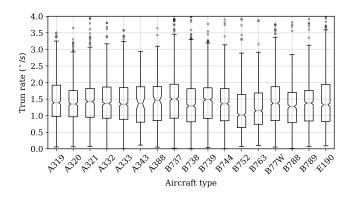
Figure 10. Distribution of estimated turn rate per aircraft type (outliers larger than 4.0 deg/s are not shown)
