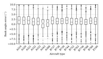
Figure 12. Distribution of bank angle estimation error per aircraft type
