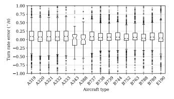
Figure 13. Distribution of turn rate estimation error per aircraft type
