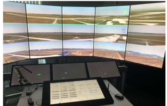
Figure 1. Multiple Remote Tower Environment at DLR Braunschweig.
