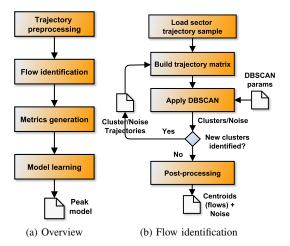
Figure 3. Methodology to build a model for OCC peak estimation with a focus on the sector flow identification process.
