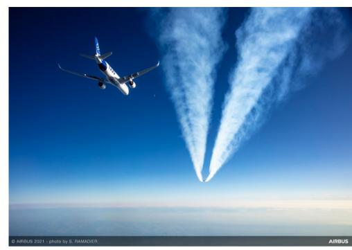
WER sees a pair of aircraft flying in formation, one around 1.5nm (3km) behind the other, allowing the trailing jet to benefit from the lift generated by the preceding aircraft's vortices, reducing the thrust required from its engines. The initial modelling suggests airlines could save between five and ten per cent of fuel per trip.
