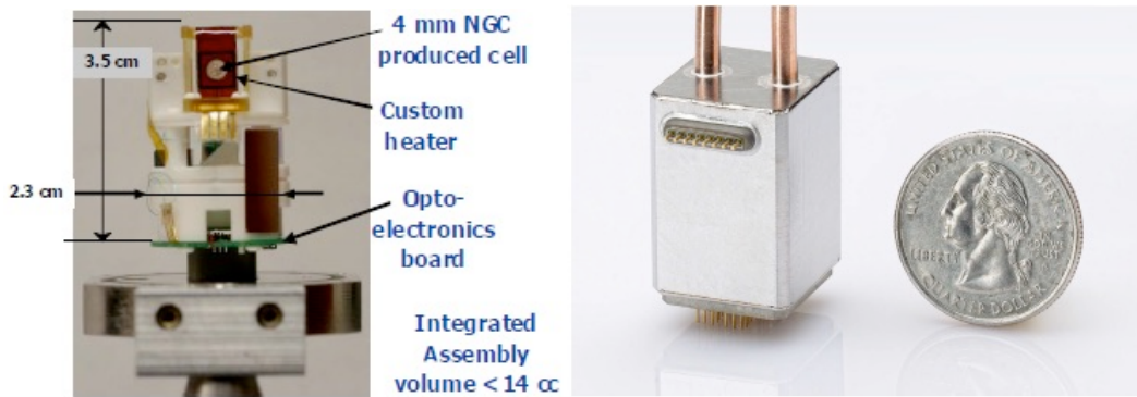
Figure 26 - Gyro internal structure, physics package of the latest version
