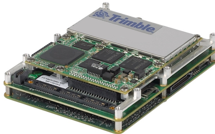
Figure 8 - The Trimble AP20, a GNSS + Inertial platform which can be used for airborne applications
