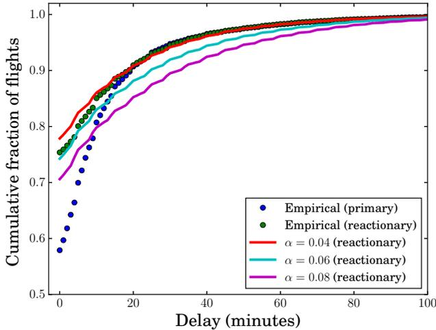
Fig. 2. Cumulative distribution of reactionary delays for the 20th of June 2013.
