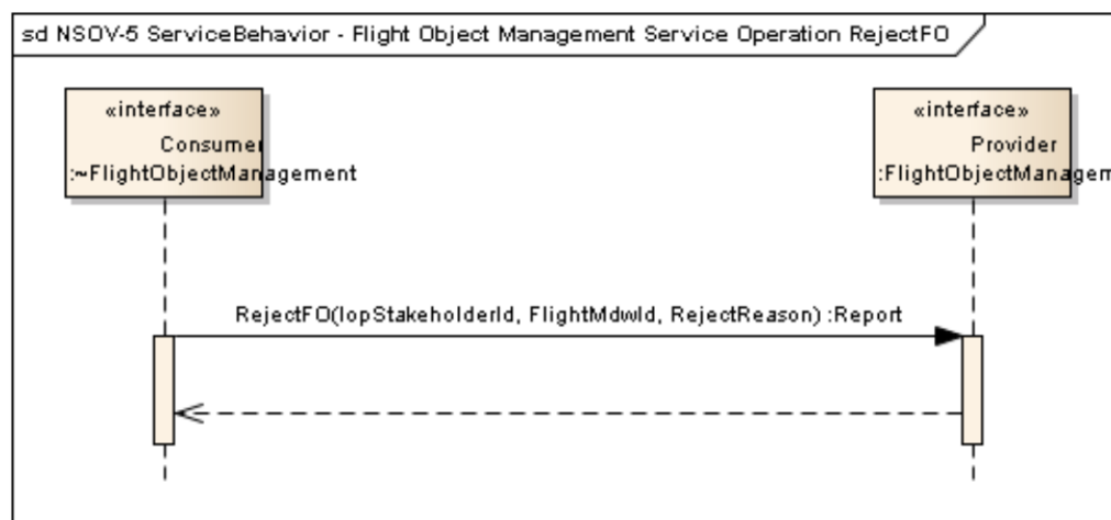
Figure 3-9: Flight Object Management Interface: RejectFO operation Behaviour
