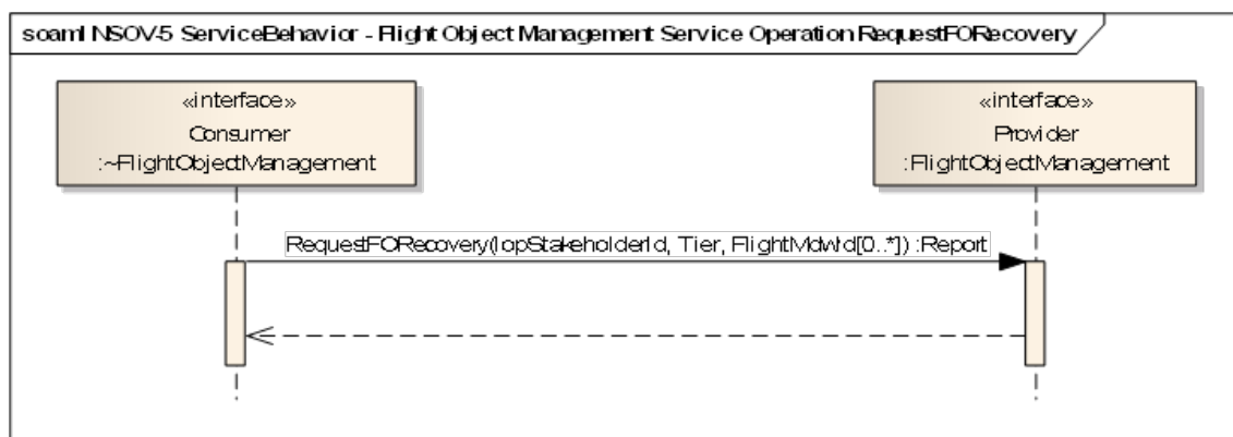
Figure 3-11: Flight Object Management Interface: RequestFORRecovery operation Behaviour
