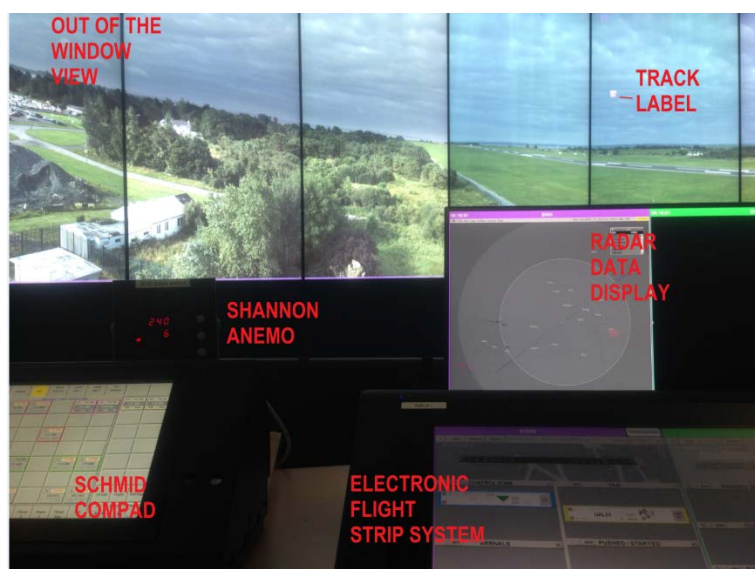
Remote Tower single working position.
