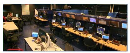
Figure 6-2: View of NARSIM Radar Controller Working Positions
